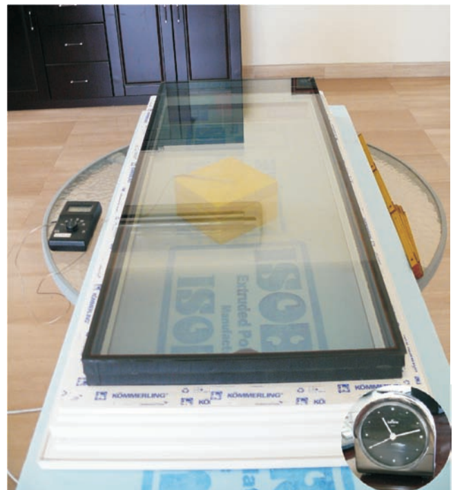
Preparation with window frame on Styro foam, heater, and thermometer
