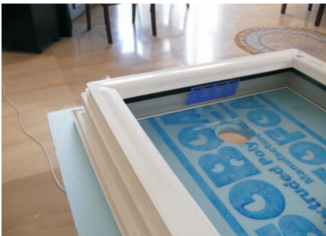
The test after approx. 2,5 h Plastic deformation on the frame from the temperature
