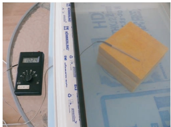
Preparation with window frame on Styro foam, heater, and thermometer
